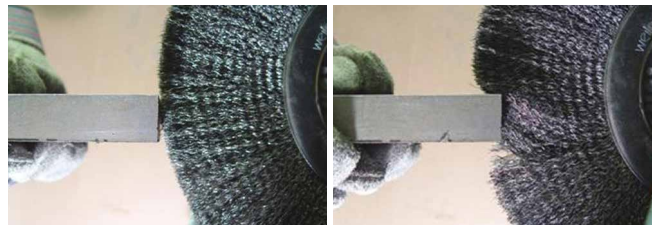
Correct Wire Tips Doing the Work
